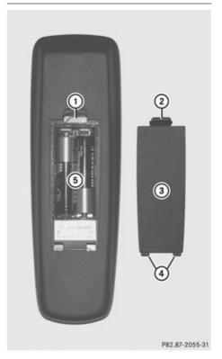
The remote control contains two batteries of size AAA, 1.5 V.
