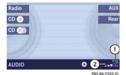
Time display with ignition on and mobile phone inserted
