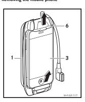
1. Slide the locking tab (6) upwards and remove the mobile phone (3) from the cradle (1).
