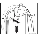
Press the release button (7), slide the cradle (1) downwards and remove.
